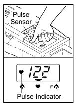
**detected.** Next, raise your thumb slightly until the heart-shaped indicator in the calories/pulse/fat calories display flashes **steadily**. Hold your thumb at this level. After a few seconds, three dashes will appear in the display and your pulse will be
